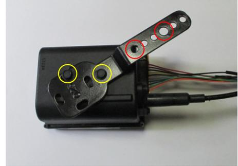
Attach the ECCS mounting bracket (Red circle holes) to the bottom of the battery carrier using 5/16"-20 x 1/2" bolts w/lock washers (bolt heads in the battery carrier drain channel).
