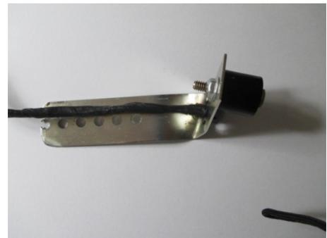
Mark the bolt-hole locations and drill small pilot holes. In the cabin, enlarge the pilot holes to 13/64" and tap for a 1/4"-20 thread. If you are doing this work without help, the threaded holes will act as another set of hands. These holes will be approximately 14" behind the automatic shifter casing. Use low-profile screws to minimize interference. Drill and tap another 1/4" hole approximately 4" behind the shifter casing for an under-carriage wire bracket.
