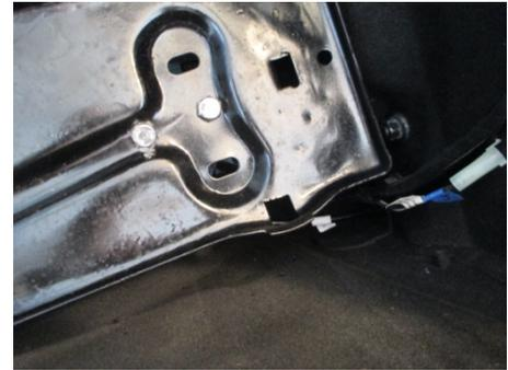
Remove the wiring-harness-through-cowl-grommet-retainer and create another hole in the grommet to fit the ECCS wiring harness. Insert the ECCS wiring harness through the grommet and into the cabin. Reinstall the grommet and retainer.
