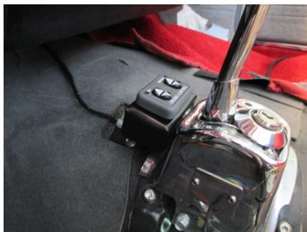
space for the carpet to slide under the mounted DMSC. A template is provided on the last page. The wiring will route under the carpet, following the transmission tunnel center and exit where the cross-dash support bars bolt to the firewall. From the cabin side of the wiring-harness-through-cowl-grommet, route the ECCS harness to the cross-dash support bar and use tie-straps to secure the harness to the left-side of the support bar.
