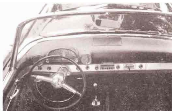
INSTRUMENT PANEL follows style of the 1954 Ford, with a tachometer (left) and sweep-second clock added. Floor shift lever controls hydramatic drive. Visibility is superb.
